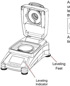
Adjust the leveling feet of the Moisture Analyzer until the air bubble in the indicator is centered. The level indicator is located under the cover towards the rear of the Moisture Analyzer.
